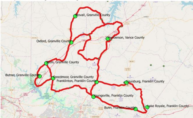
The blue points below are telecom and service locations provided by the Kerr-Tar COG. By connecting all of the High-Density population areas, most of those sites can be connected within these rings. Laterals and connections to the backbone can be run later, or the backbone can be expanded as needed.
